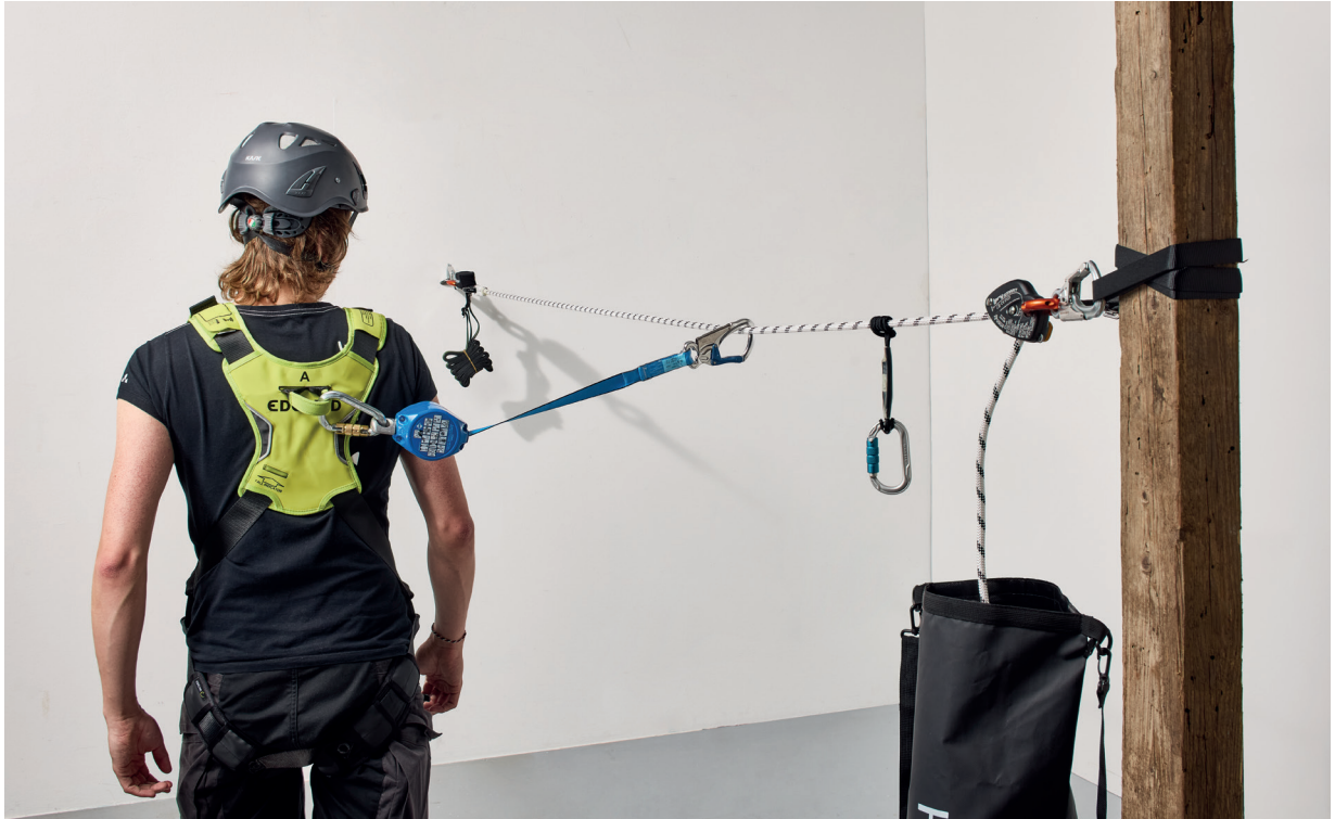
Fig. 7: Lifeline is tensioned at the height of the back eyelet with retractable type fall arrester
