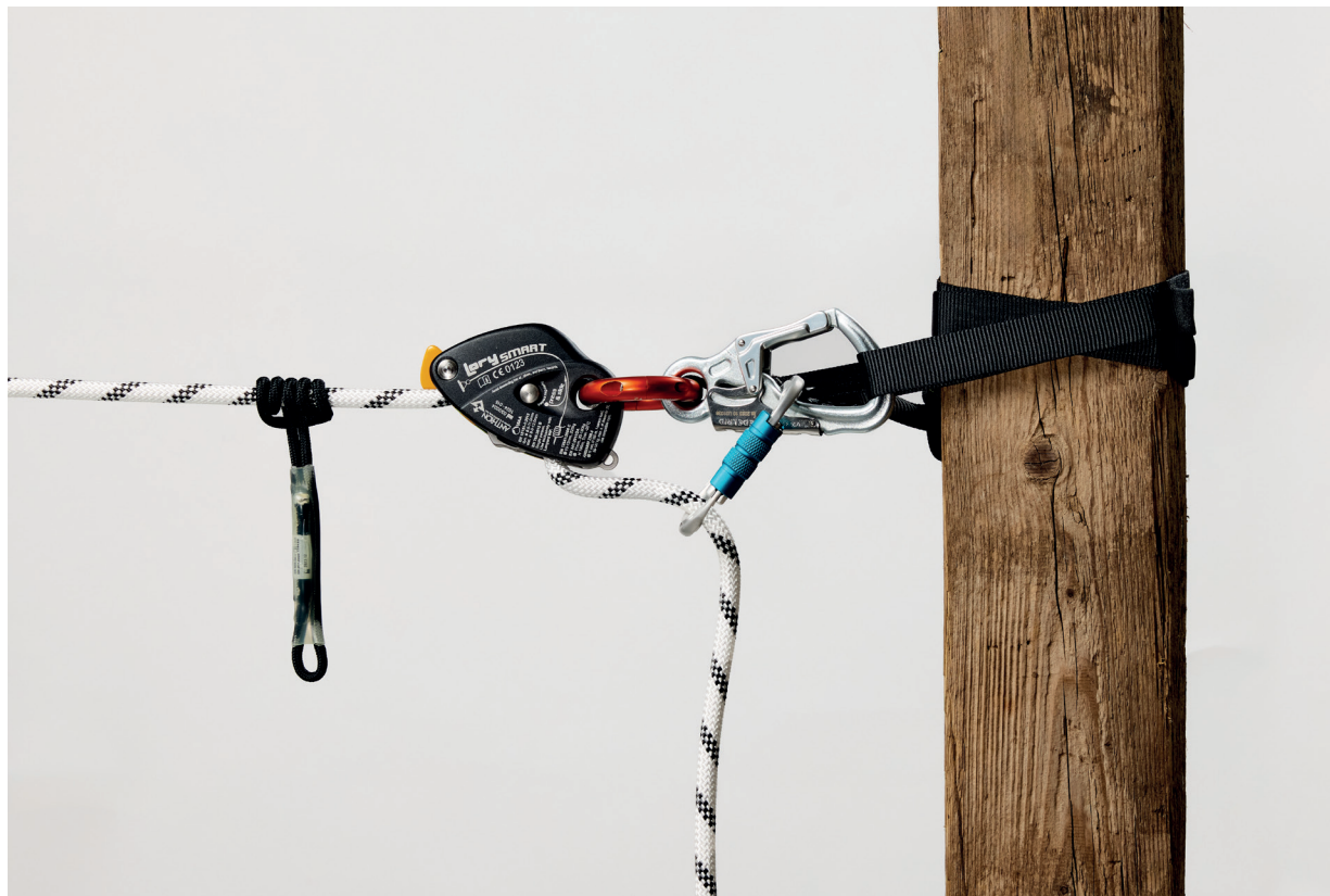
Fig. 11: Carabiner is hooked into the vertebra and closed
