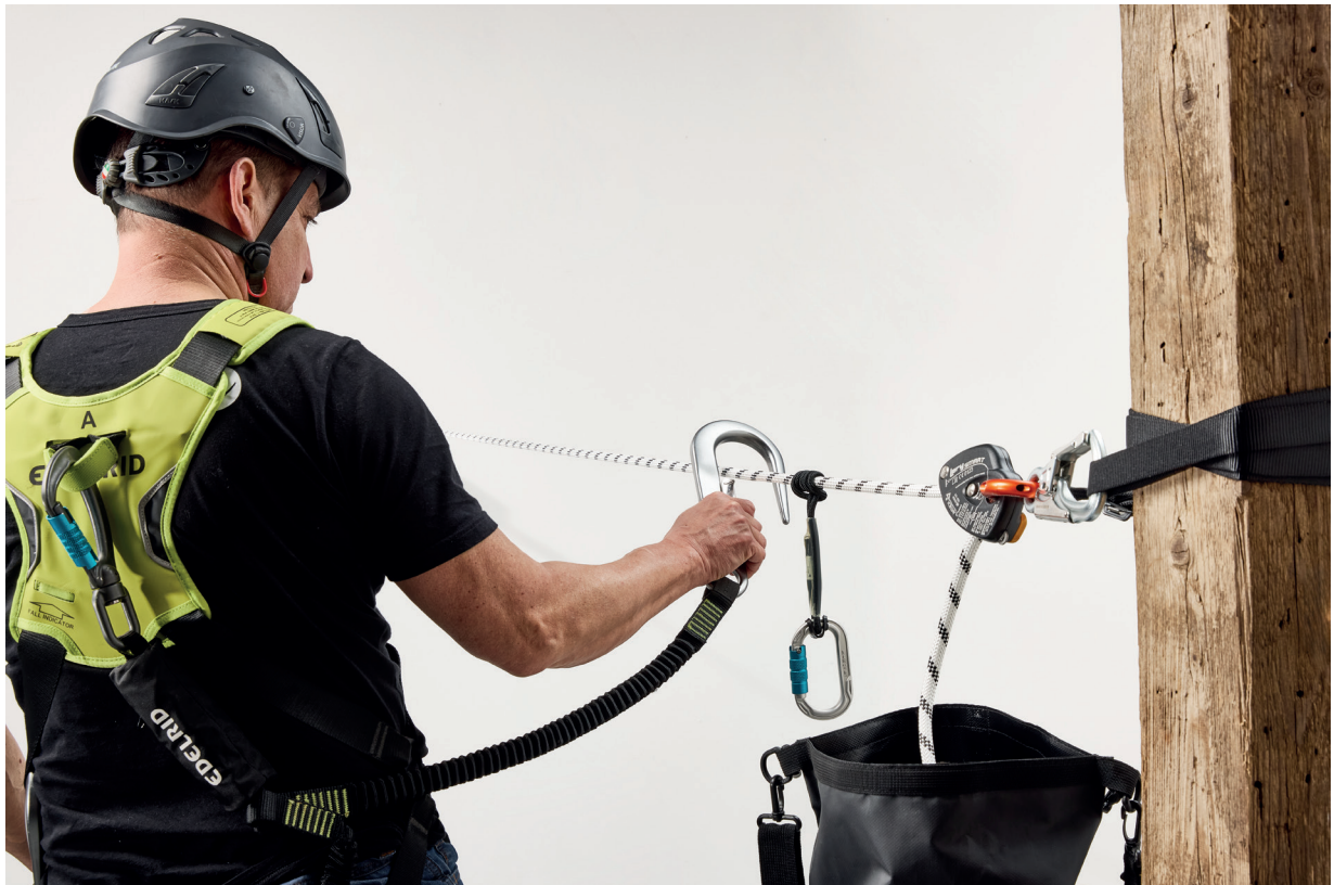
Figure 8: Attachment to lifeline with lanyard
